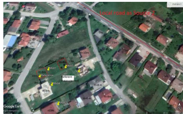
Figure 2. Modeling scheme for stable and local road as line source with measurement positions as reference and new objects and additional positions.
