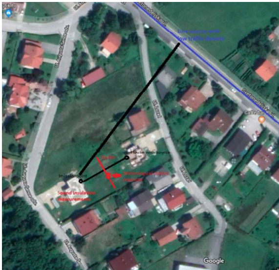
Figure 1. Measurement situation for stable source and local road with location of sources and imission points).
