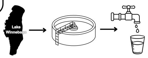
The water is lime softened and filtered through granular activated carbon for turbidity removal. Ultraviolet Light is used as a disinfection process for Cryptosporidium. Fluoride is added for dental health. Finally, chlorine disinfection provides safe, drinking water throughout the distribution system and to your faucets.
