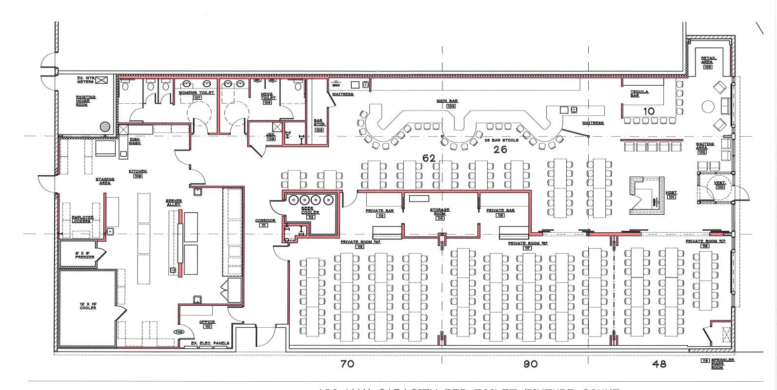
450 MAX CAPACITY PER TOILET FIXTURE COUNT 306 SEATING CAPACITY
