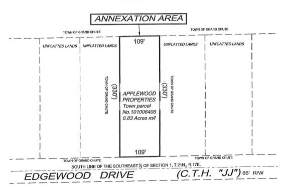
BEARINGS ARE REFERENCED TO THE WISCONSIN COUNTY COORDINATE SYSTEM, OUTAGAMIE COUNTY, SOUTH LINE OF SE 1/4 SECTION 1, T.21N., R.17E.; recorded to bear N89\*14\*49\*E
