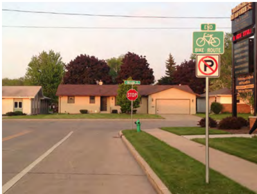
Facilities ending without further information can create gaps at intersections
