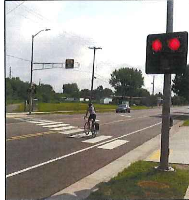
Figure 19: Pedestrian Hybrid Beacon ("HAWK")
