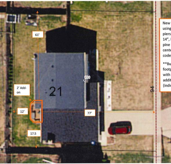
New 12'x16' deck build, using (5) 50/50 diamond piers. Height off grade is 14", KDAT treated southern pine frame (2x10, 16" on center). Includes 1 stair and code compliant railing.
