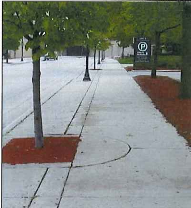
Figure 14: Sidewalk A sidewalk is a dedicated space for pedestrians adjacent to a street. Most streets in Downtown Appleton have sidewalks. A 5-foot sidewalk is typical in residential neighborhoods; in commercial areas, sidewalks can be much wider than 5 feet to accommodate additional pedestrian traffic and street furniture.
