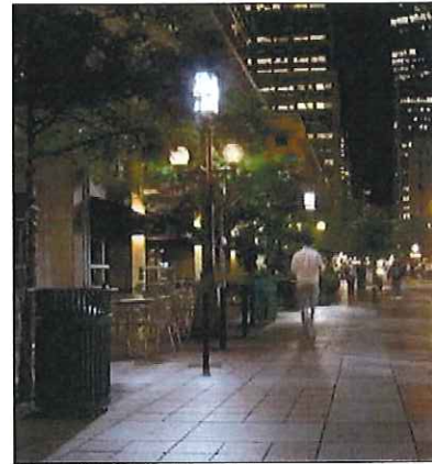
Figure 25: Pedestrian Lighting Standard street lights often do not provide adequate lighting of pedestrian areas including sidewalks. In areas with significant pedestrian use, anticipated pedestrian use, or concerns about safety, pedestrian-scale lighting should be installed. Pedestrian-scale lighting focuses light on pedestrian areas including sidewalks and shared use paths, often using light fixtures that are lower to the ground than traditional street lights. Pedestrian-scale lighting often uses decorative poles that can enhance the aesthetics of a street, or provide a historic appearance in historic areas.
