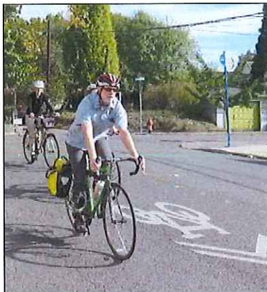
Figure 33: Bicycle Boulevard (Neighborhood Greenway) A bicycle boulevard is a street with low motorized traffic volumes and speeds designated to provide priority to bicyclists and neighborhood motor vehicle traffic. Bicycle boulevards may simply have signs and shared lane markings, or may include traffic calming elements including speed humps, traffic circles, chicanes, or traffic diverters. Bicycle boulevards benefit neighborhoods by reducing cut-through traffic and speeding without limiting access by residents. Recommendations for bicycle boulevards in this plan do not include guidance for specific treatments.
