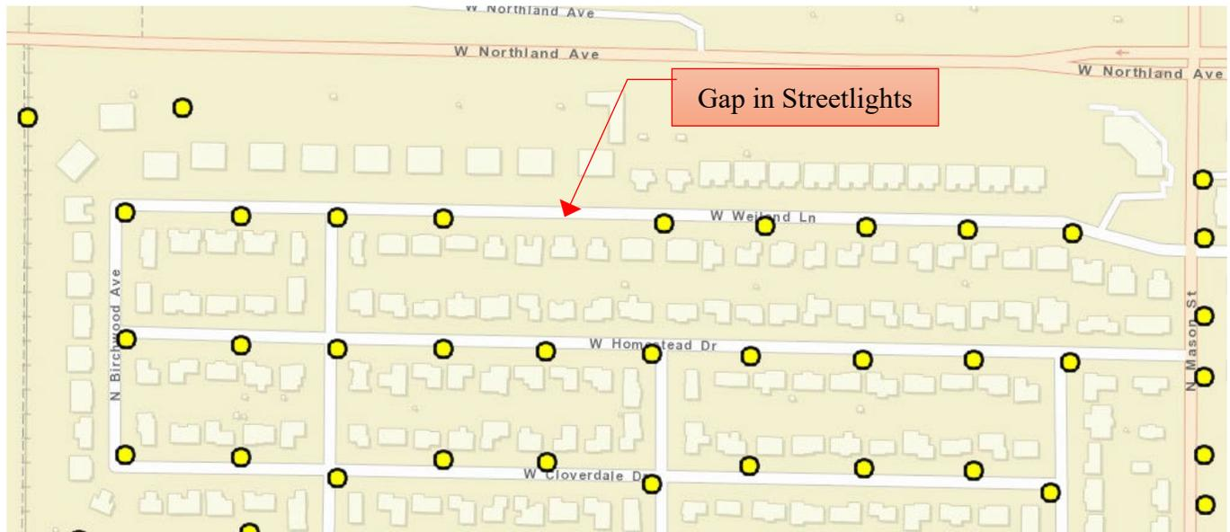
WE Energies was asked to prepare a design and cost estimate to add a new streetlight that fills the gap, matching the style and spacing of existing streetlights. We propose a wood pole with light be added between the properties of 1617 and 1625 W. Weiland Avenue. The power would be fed underground from the existing power pedestal along the back lot utility easement, same as other lights on the street.
