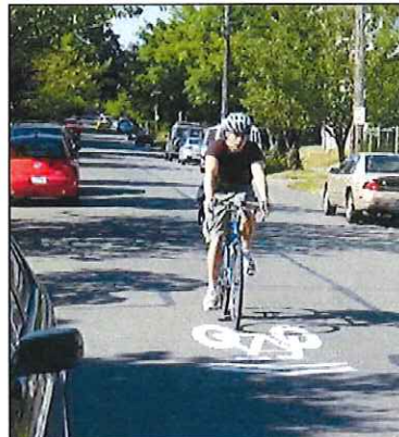
Figure 34: Shared Lane Marking (Sharrow) Shared lane markings, sometimes called sharrows, are used on streets where bicyclists and motor vehicles share the same travel lane. The sharrow helps position bicyclists in the most appropriate location to ride. It also provides a visual cue to motorists that bicyclists have a right to use the street.
