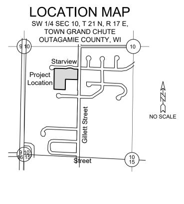
Bearings are referenced to the West line of the Southwest 1/4, Section 10, T21N, R17E, assumed to bear N00°50'37"W, base on the Outagamie County Coordinate System.
