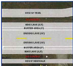
New Roadway Configuration (to be implemented in 2019)
