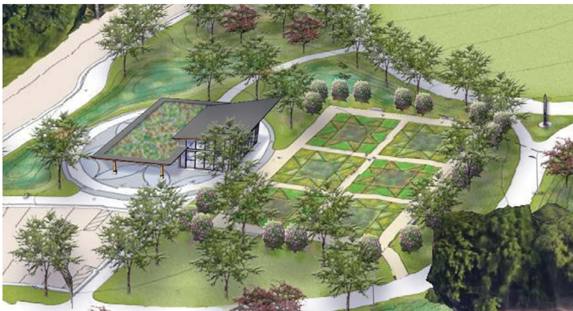
Pavilion/Restroom with potential green roof (sedum garden to match quilt pattern of the plaza below)
