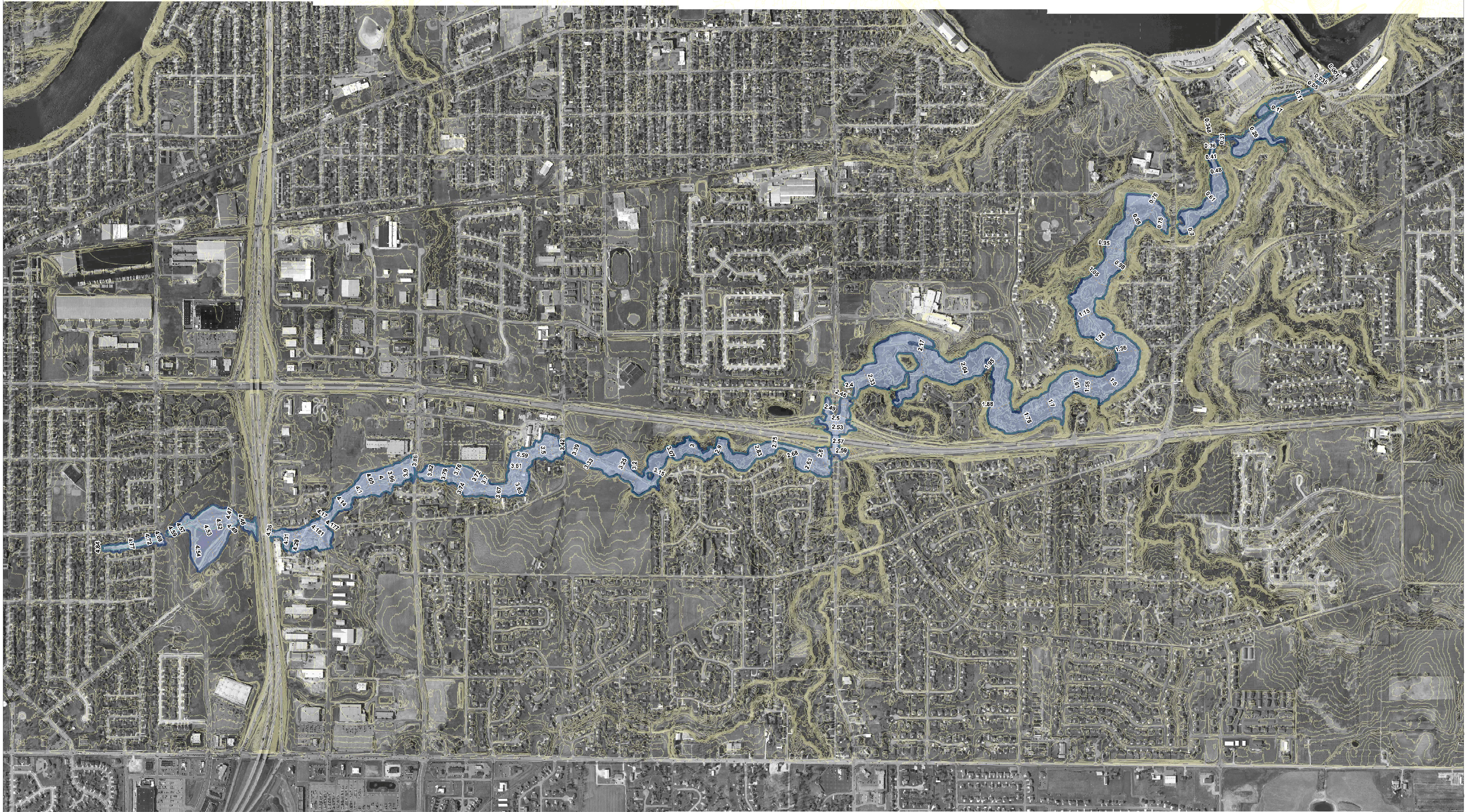
95346 July 2007 Figure 2 City of Appleton Kensington Pond Dam Break Analysis Hydraulic Shadow Legend FIS/Flood Study Cross Sections Hydraulic Shadow Contours 0 250 500 1,000 1,500 2,000 Feet N
